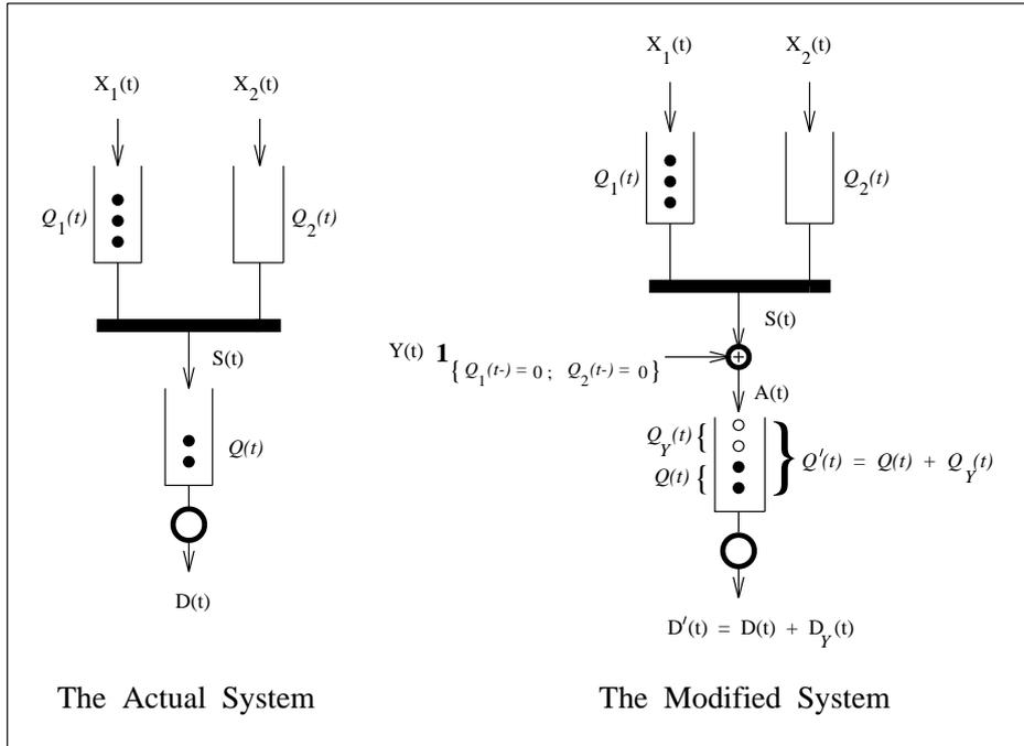
Figure 3: The SM/M/1 queue (on the left) with two synchronized independent Poisson inputs and an exponential server. On the right, the modified system used to analyze the SM/M/1 queue is shown, in which “ghost tokens” (represented by empty circles) are injected to the service queue.
