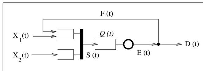
Figure 6: Feeding all synchronization buffers by non-feedback flows prevents stalling of the synchronization node.
