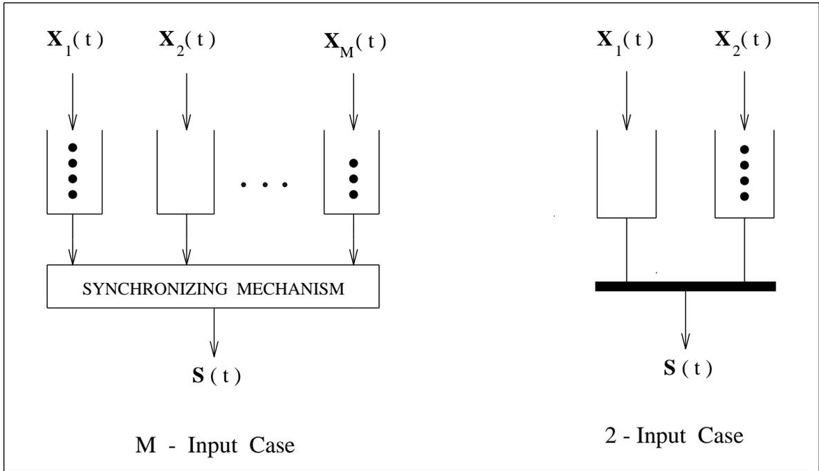
Figure 1: Synchronization of point processes. At least one queue is always empty.
