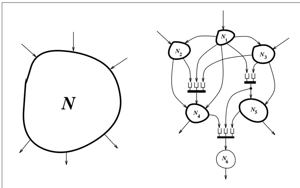
Figure 7: A network with an acyclic synchronization skeleton. Local networks of only service nodes may be non-acyclic.
