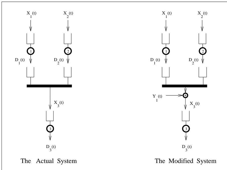
Figure 4: Interfacing service queues through synchronization ones. In the modified system the controlled flow  $\mathbf{Y}_1(t)$  injects “ghost tokens” into the flow  $\mathbf{X}_3$ , making the latter Poisson by accounting for the deficit of actual tokens.
