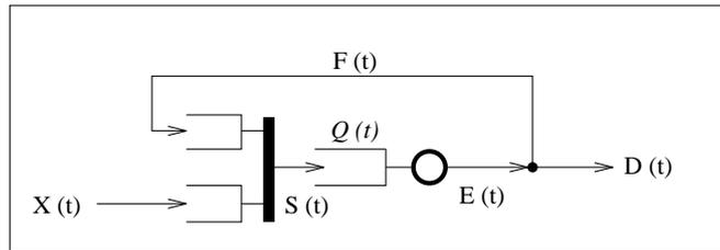
Figure 5: A simple network with feedback of tokens to the synchronization node. The node will eventually stall.
